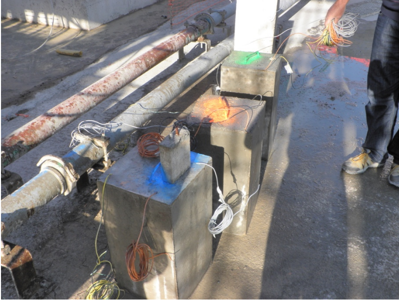
Image 2: Pilot specimens with the monitoring systems installed
